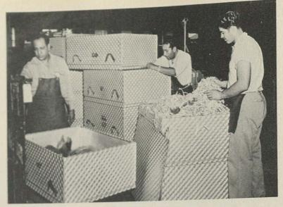
Weighing in and packaging new type shipping containers for air shipment.
