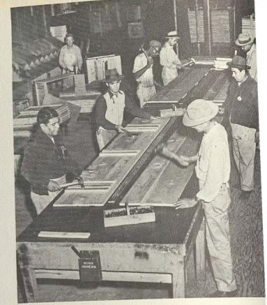
Speedy nailing crates together ready to be quickly assembled by sections.
