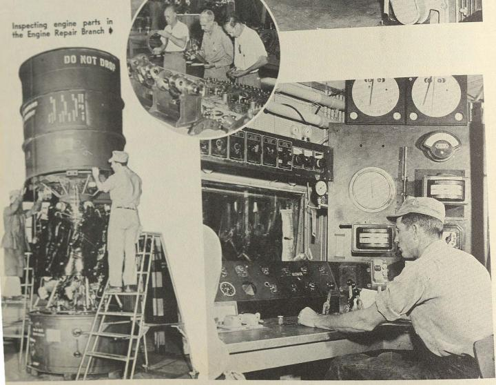
B-36 engine is placed in shipping can after being overhauled at Kelly AFB
