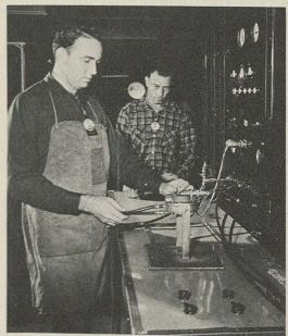
Pressure switch testing.
