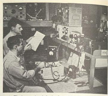
Final operational check of very high frequency radio receiver carried in most air force aircraft.
