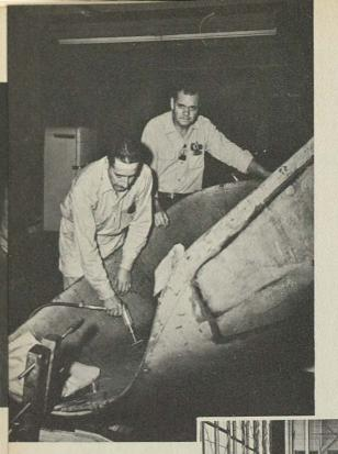
Replacing a section of skin on a T-6 wing under the supervision of Mr. Phil Karrer, left, Chief of Wing and Surface Section. Bldg. 312.
