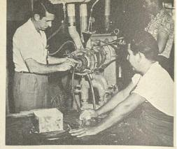
Bldg. 329, extrusion of rubber tubing.
